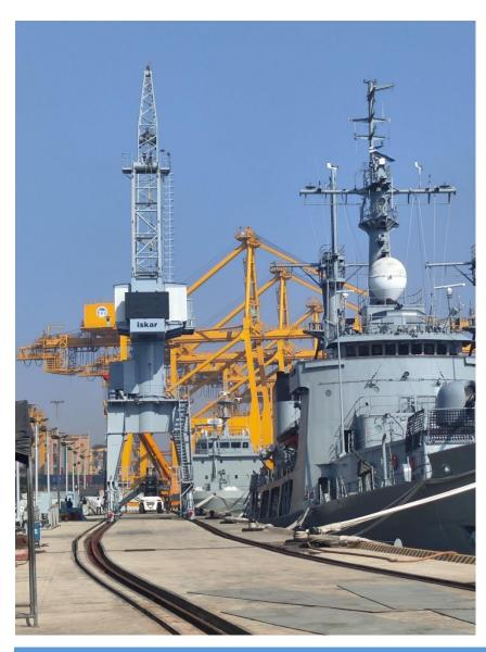
CSD (Issa Khan) is Bangladesh Navy Dockyard located in Naval base of Chittagong. As being one of the largest Naval bases of Bangladesh Navy, CSD serves as the most important base. 1 slewing jib, lattice boom hook duty slewing crane with curve travelling feature is delivered onto the new build jetty.
