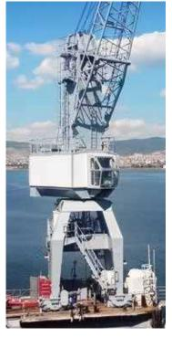
Cranes of YHV series are suitable for floating dock applications. Handling of hook loads for general ship repair and maintenance works are common operation modes. Typical of the YHV type crane design is the narrow rail span length and the feature to luff the jib down to rail level during towing of the dock on open seas. Floating dock cranes are the main power of ship repair yards and therefore shall be carefully engineered to achieve its duties.
